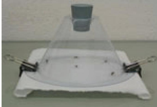
Fig 5. Cone used in cone test for mosquito repellents by WHO
