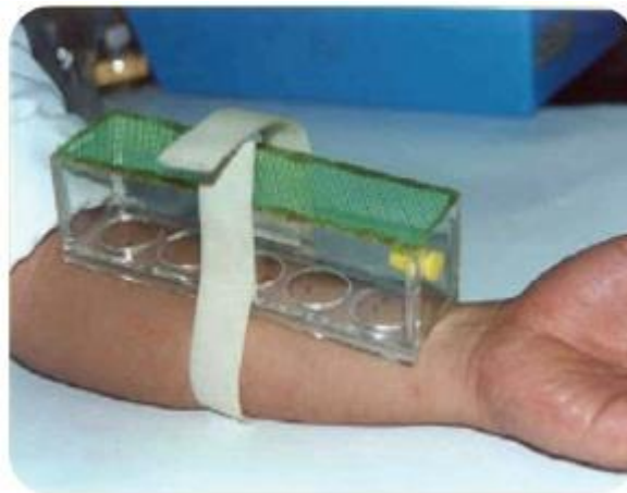
Fig 6. Test Cage method for mosquito repellents by ASTM
