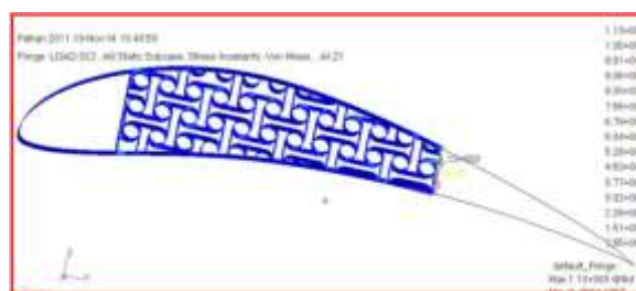
Fig. 37 von-Mises Stress at a Load of 150N
