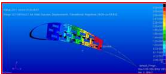
Fig. 17 Trailing Edge Displacement at a Load of 20N
