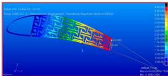
Fig. 30 Trailing Edge Displacement at a Load of 20N
