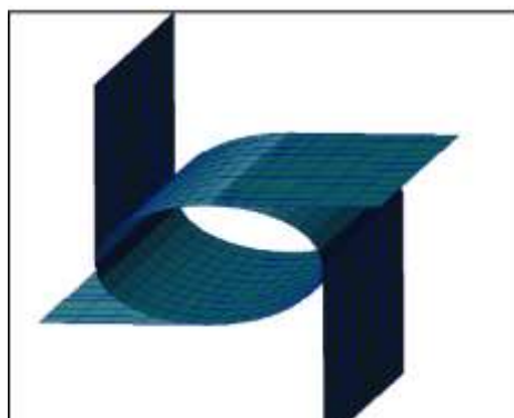
Fig 3: FE Model of the unit cell (Elliptical node & Circular node) with shell elements
