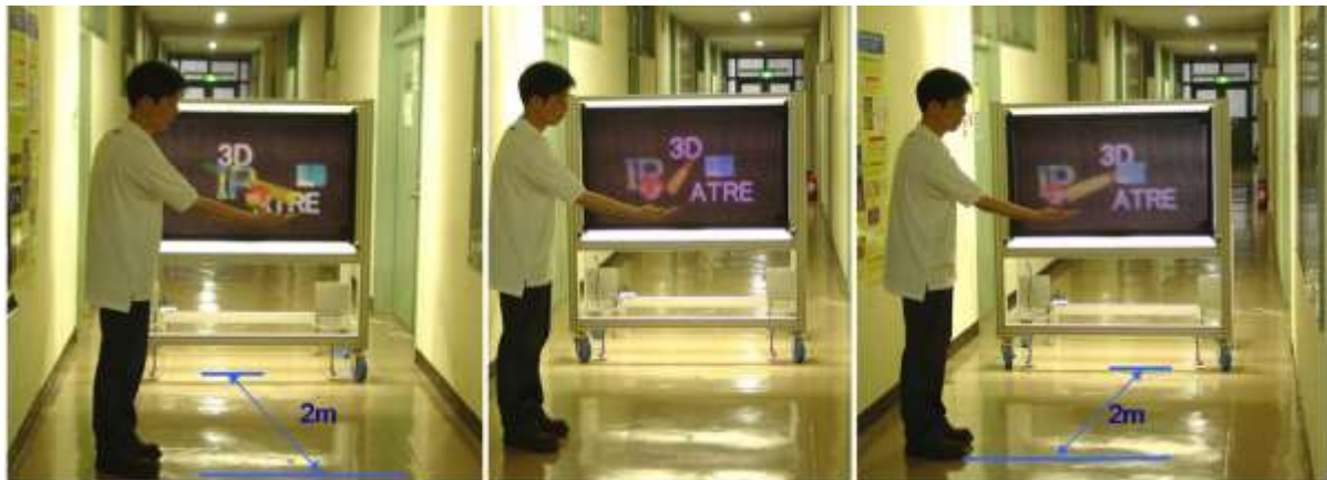
Fig. 6. 3D computer graphics image produced by the IV autostereoscopic display for distant viewing, viewed from the left to right. The club stands out in mid-air on the palm of the viewer's hand about two meters away (yellow part) and four meters inside (red and green part) the display. (See supplementary Movie, which can be found on the Computer Society Digital Library at http://doi.ieeecomputersociety.org/10.1109
