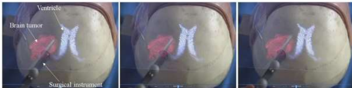
Fig 3. Images overlay of tumor, ventricle, and surgical tool onto the phantom of the human brain. The photographs show different steps of insertion of a simulated surgical instrument
