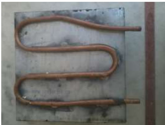
Fig 3 : Copper Tubing at rear of Absorber Plate
