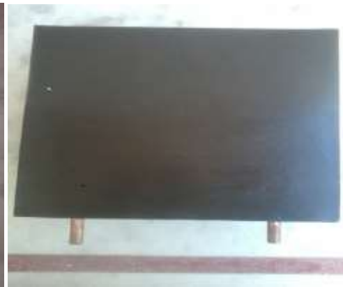
Fig 2 : Black Painted Absorber Plate
