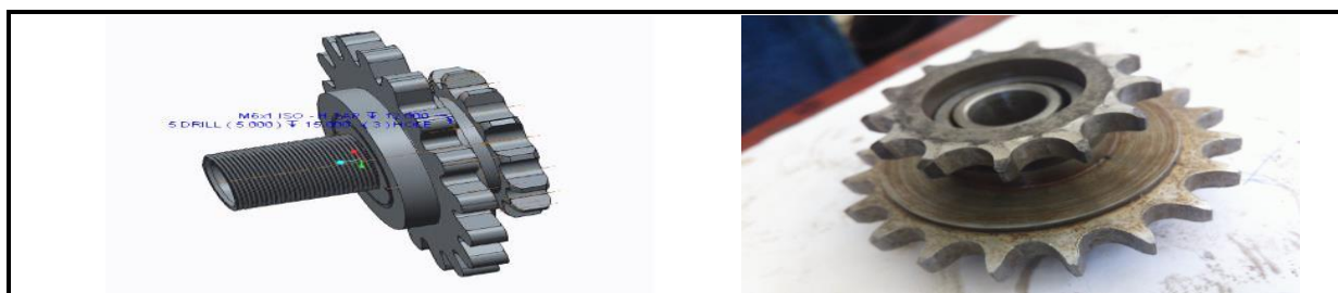
Figure 2. CAD Model and Actual Image of Compound Ratchet Sprocket
