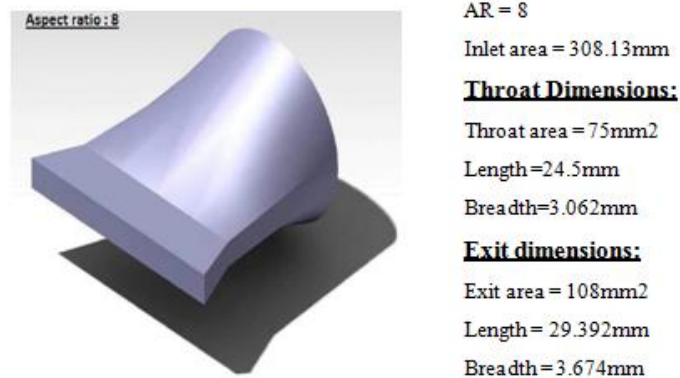
Fig. 3. Isometric view of (a) AR 2 (b) AR 4 (c) AR 6 (d) AR 8 Nozzle with design parameters
