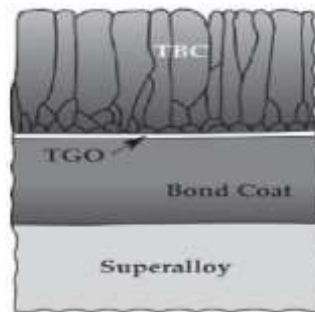
Fig 1: Diagram shows the cross section of multilayered thermal barrier coating
