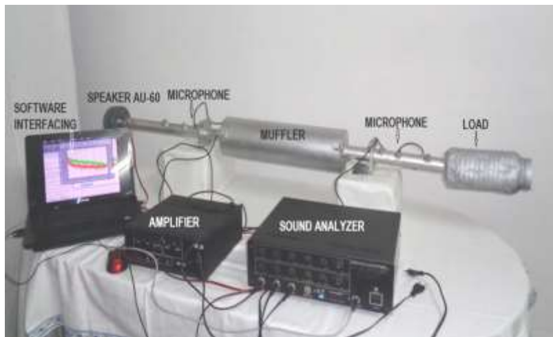
Figure 1: Muffler Transmission loss measurement setup with load
