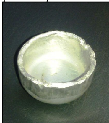
Fig. 5 Successful Deep Drawing Cup for AA 8011 of 1.5 mm thickness
