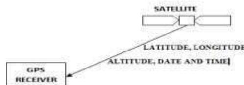
Here SR-92 GPS receiver is used as it is highly efficient and it consumes less power. Generally GPS receiver is connected to the UART as it transmits data in a serial manner.
