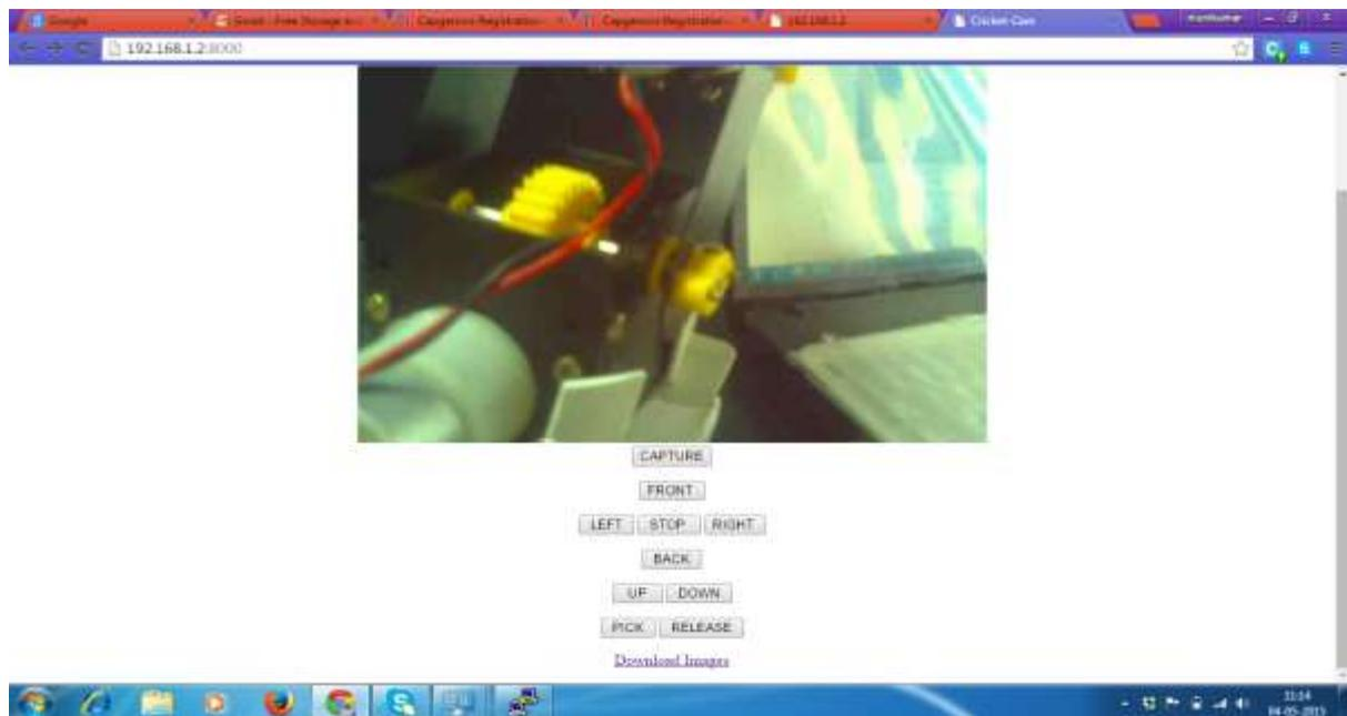
*Figure 8: Control Robotic Arm with Web Page*
