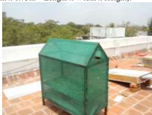
Figure 1 Solar Greenhouse Dryer
