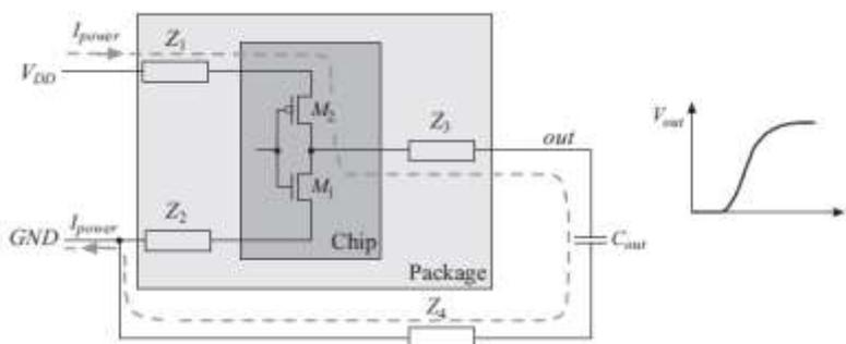
Figure 1.09: Charging of an off-chip load.
