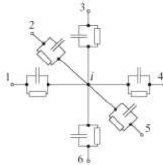
Figure 1.5: A model of the cube shaped substrate element.
