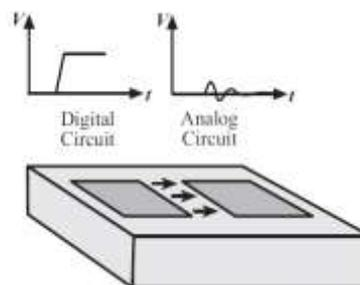
*Figure 1.1: substrate noise in a mixed-signal circuit*
