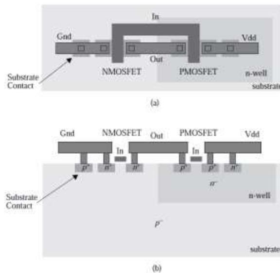
*Figure 1.11: An inverter (a) seen from above, and (b) seen from a vertical cut.*
