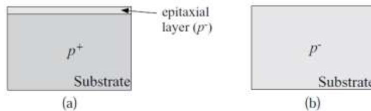
Figure 1.2: (a) Heavily doped substrate, and (b) lightly doped substrate.
