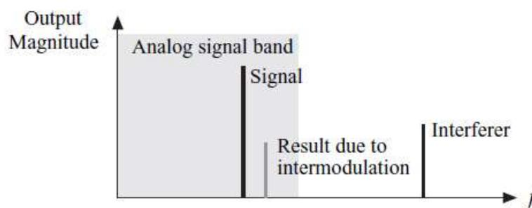
Figure 1.15: Example of intermodulation of a signal and an interferer where a resulting frequency component falls into the analog signal band
