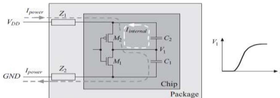
Figure 1.07: Charging of an on-chip node in a digital circuit
