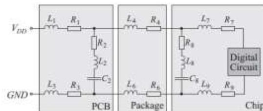
*Figure 1.10: A model of the power supply lines of a digital circuit.*
