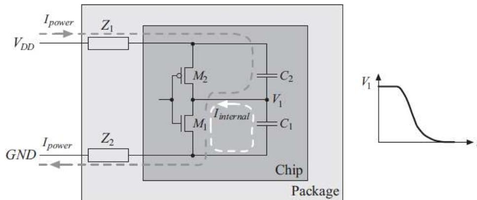
Figure 1.08: Discharging of an on-chip node in a digital circuit.
