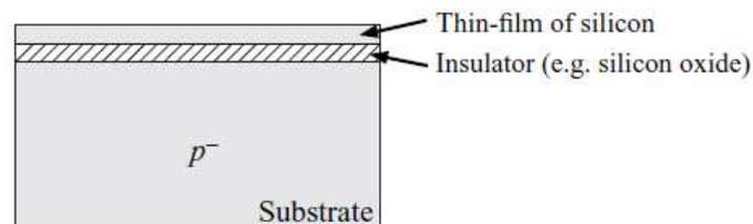
Figure 1.3: Silicon-on-insulator (SOI) substrate
