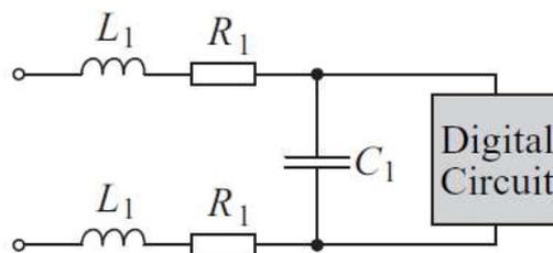
Figure 1.06: A simple model of the impedance in the power supply lines of a digital circuit.
