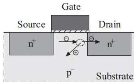
**Figure 1.12: Illustration of impact ionization in an NMOSFET**
