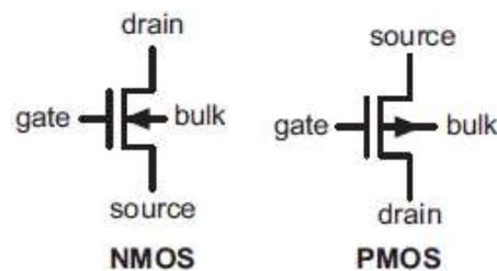
Figure 1.14: Symbols for NMOS and PMOS transistors.
