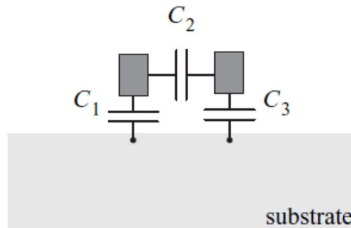
**Figure 1.13: Capacitive coupling of two adjacent interconnects.**
