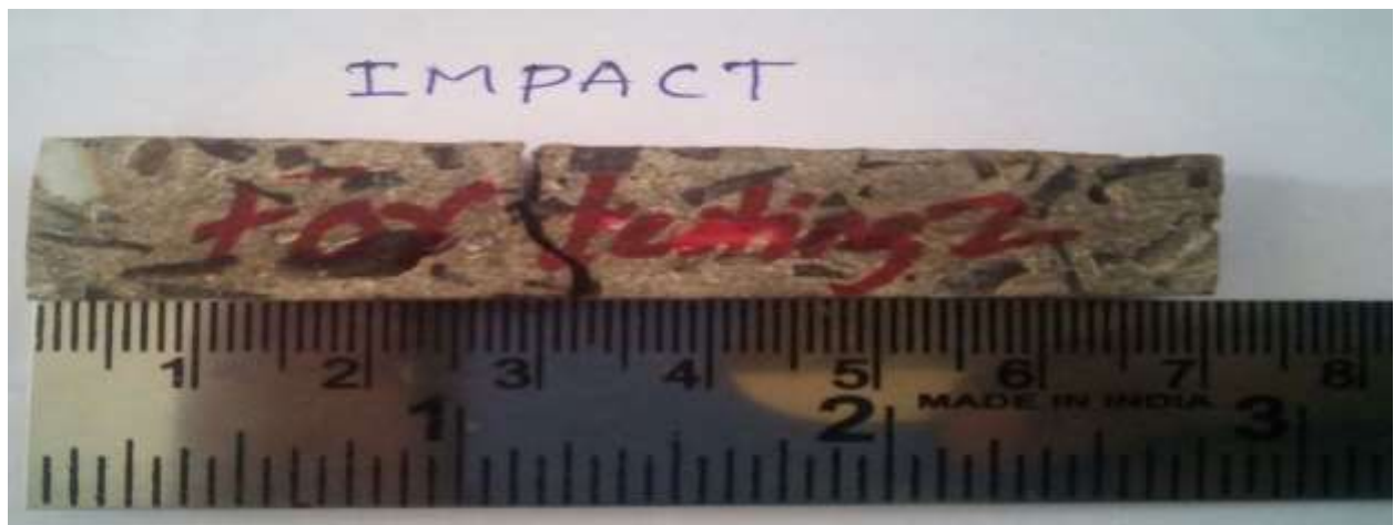
Fig. 4 Cracked DRFP composite specimen under impact test.
