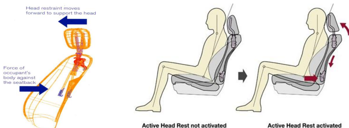
Figure 7 Working of Active Head Rest System
