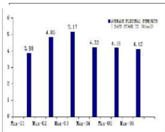
Figure 5. Flexural Strength in N/mm 2 at 7 days
