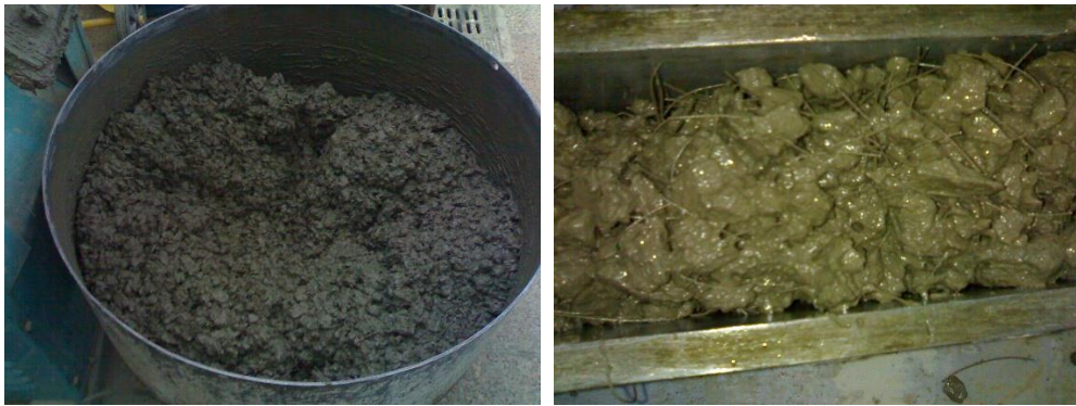
Fig. 3: RSFRC ready to be casted (Left) and casting a beam sample (Right)
