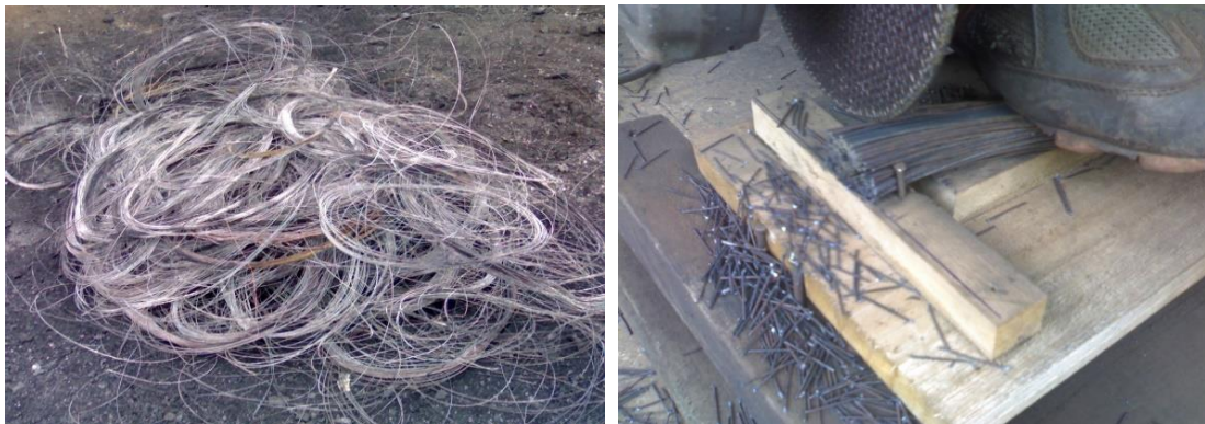
Fig 1: Extracted steel fibers from used tyres (Left) and Cutting the recycled steel fibers (Right)
