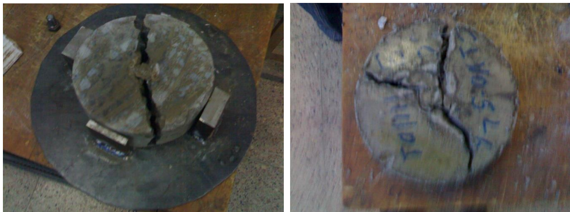
Fig. 16: Ultimate failure of a plain sample (Left) and Ultimate failure of RSFRC sample (Right)
