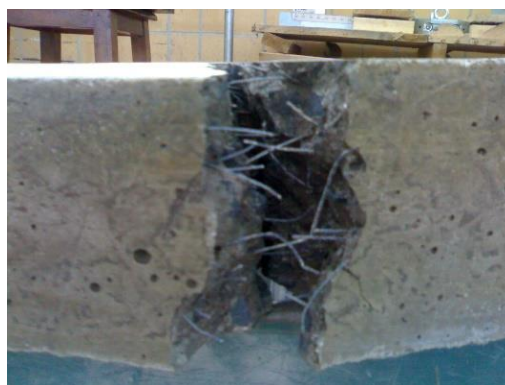
Fig. 7: A beam sample failing in flexure by fiber pull-out
