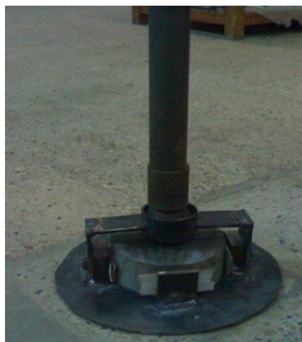
Fig. 6: Marshal hammer used for the Impact Test
