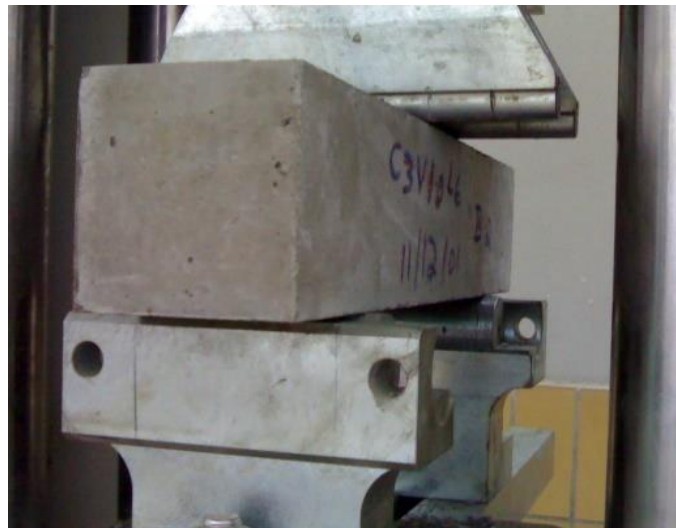
Fig. 4: Test set-up for two-point loading
