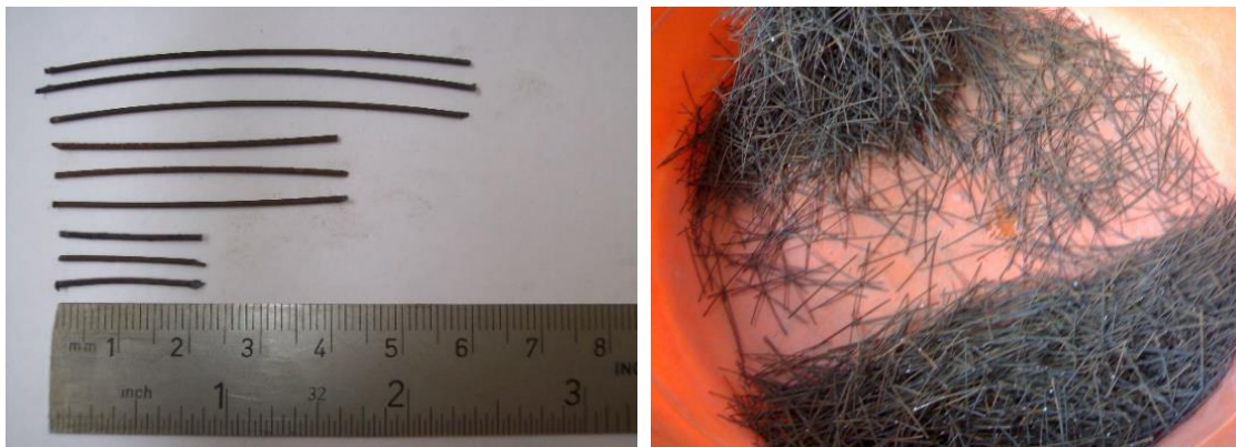
Fig 2: Preparing the recycled steel fibers into the required length (Left) and Steel fiber ready for the mix (Right)
