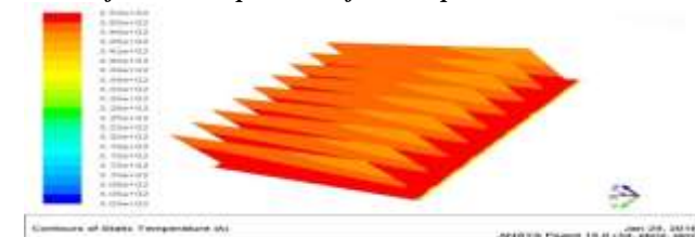
Contours of Static Temperature of the Trapezoidal Heat Sink at 353K
