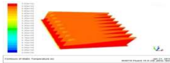
Contours Of Static Temperature Of The Rectangular Heat Sink At 363K
