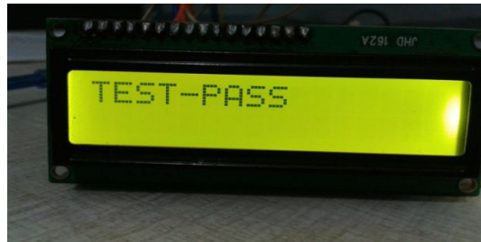
Fig 7: Output of Automated testing of Energy Meter showing test is PASS.
