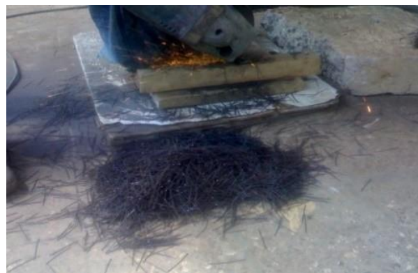
Figure 3. Cutting the steel fibers into the desired length
