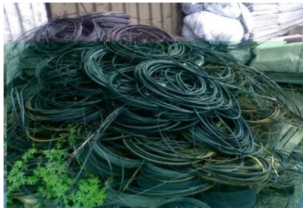
Figure 1. Defective bead wires readied for the pyrolysis process
