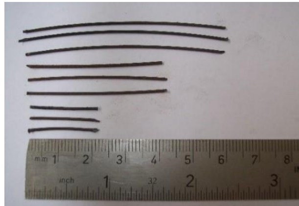
Figure 4. The three lengths of steel fibers used in the mix
