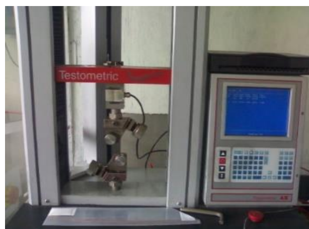
Figure 5. Testometric Machine for tensile strength of steel fiber
