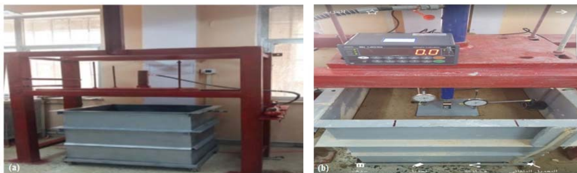
Figure 4 (a) Steel frame and axial loading; (b) Full model details.
