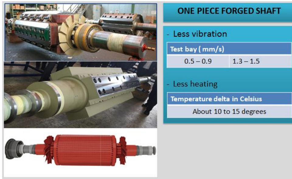
Figure 6: Rotor construction
