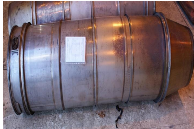
Jet Pipe To Be Reconditioned
