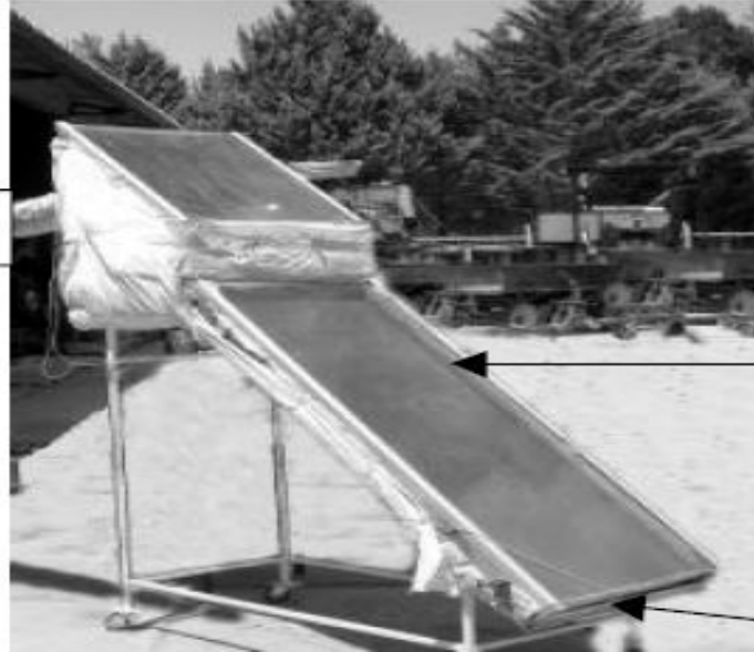
Fig. 2.9 Pictorial view of mixed mode passive dryer [12]
