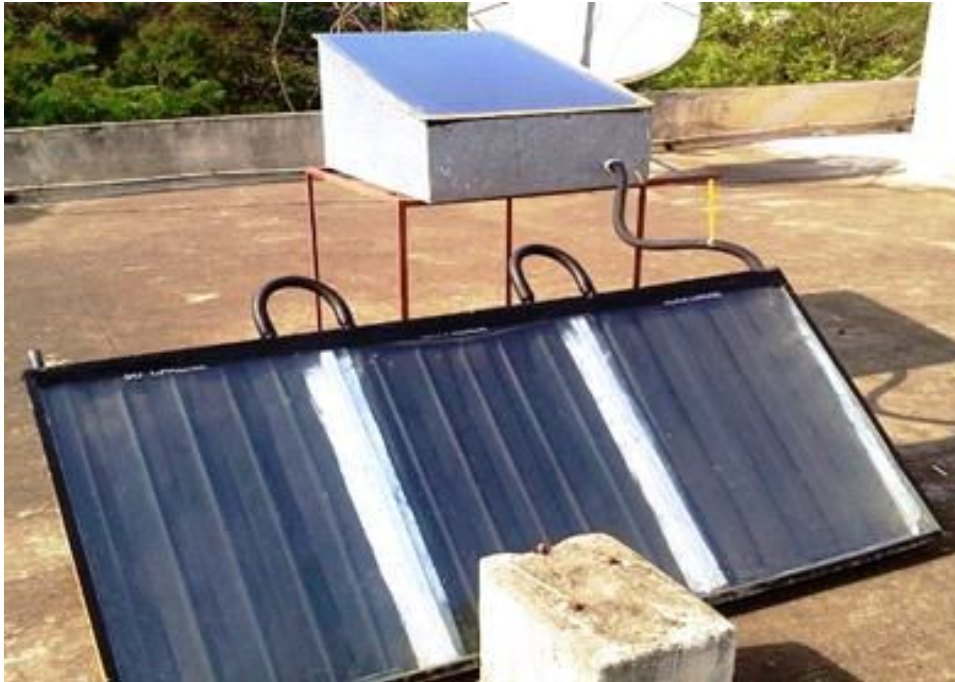
Fig. 2.8a Free convective mixed mode dryer with flat plat collector [11]
