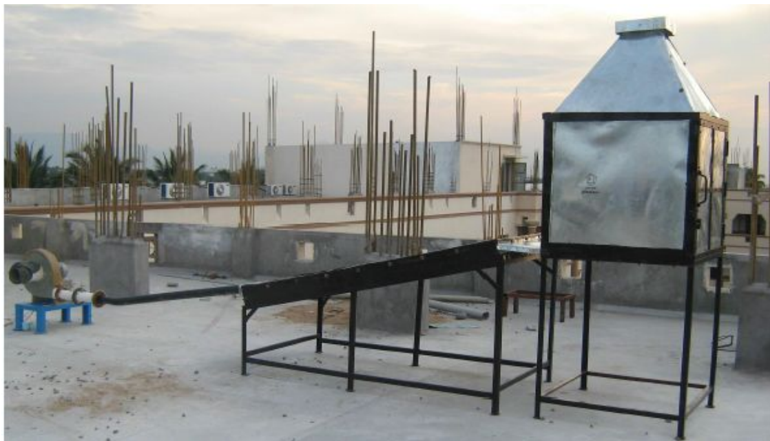
Fig. 2.4b Pictorial diagram of indirect mode dryer with heat storage materials.[7]
