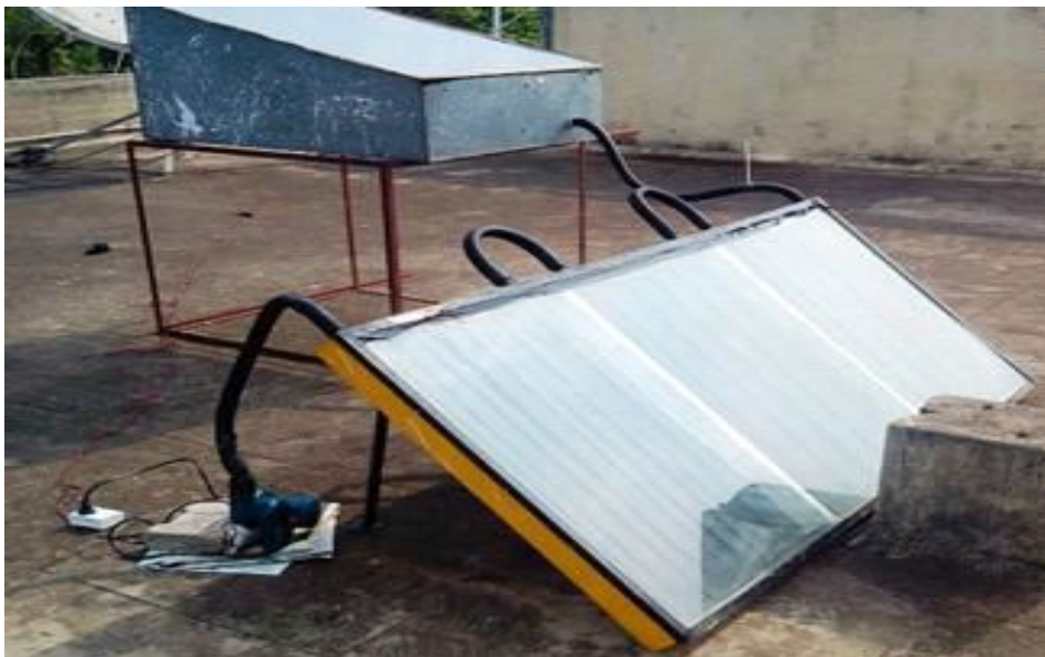
Fig. 2.8b Forced convective mixed mode dryer with flat plat collector [11]
