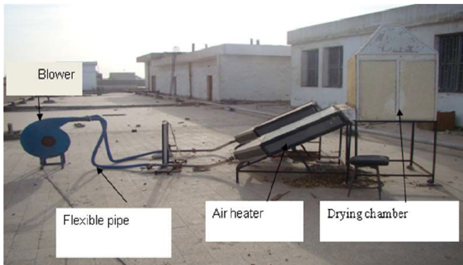
Fig. 2.6b Pictorial diagram of indirect mode dryer with and without heat storage [9]
