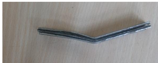
Fig. 6. Flexural test -specimen after failure
