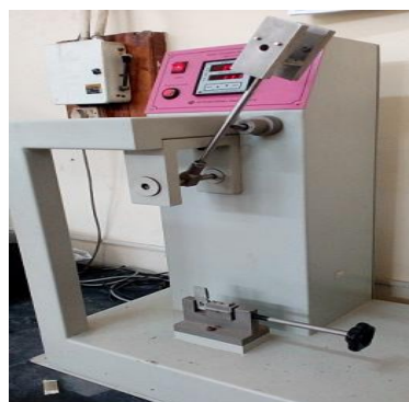
Fig. 7. Impact test -specimen loaded in the Impact Tester
