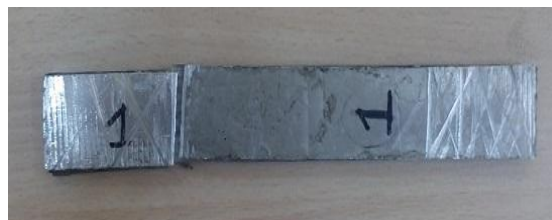
Fig. 4. Tensile test- specimen after failure
