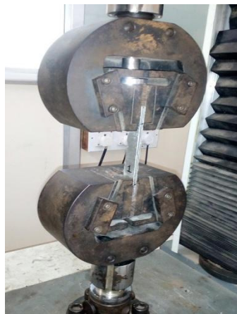
Fig. 3. Tensile test- specimen before failure
