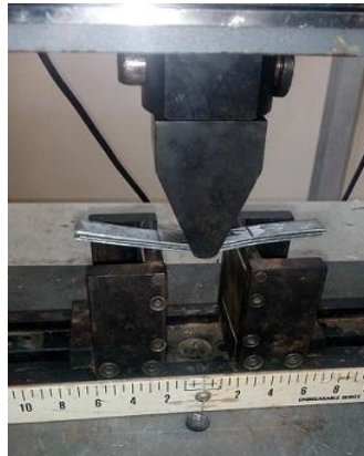
Fig. 5. Flexural test setup in universal testing machine
