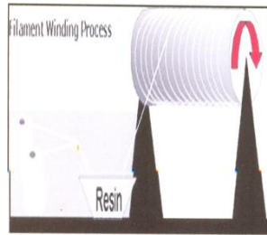
Fig.1.4 Filament winding process
